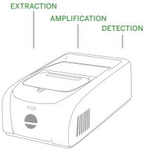
The compact FilmArray instrument performs extraction, amplification, and detection in a single for higher throughput.
